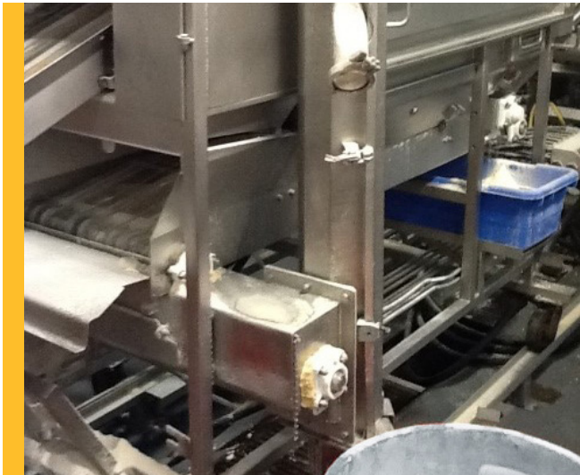
E-Z Kleen bearings replaced every bearing on the bread crumb machines, becoming the standard throughout the facility.
