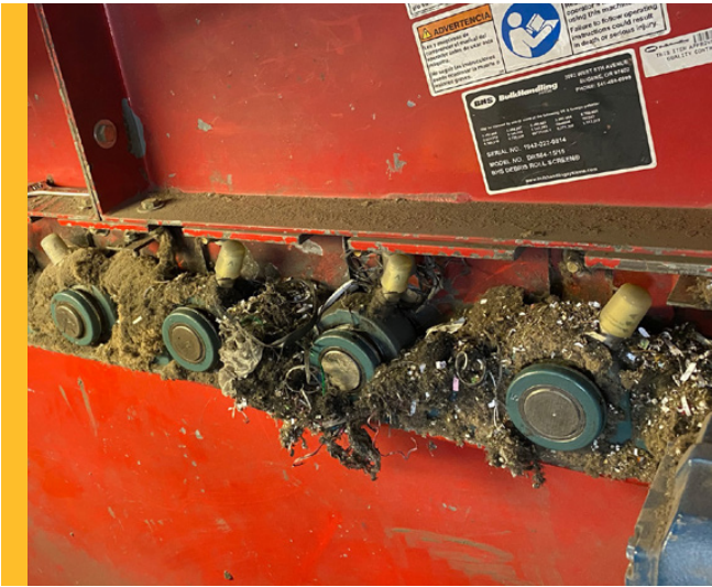
Steel discs are mounted to shafts secured on either side of the DRS deck with mounted spherical roller bearings—critical to keeping the DRS in smooth operation.
