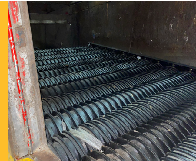
A DRS is a separation device featuring rotating steel discs that break and remove glass as well as other small debris.
